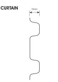
0.5mm continuous brake pressed steel curtain.
