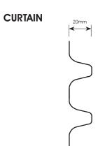
0.5mm continuous brake pressed steel curtain.
